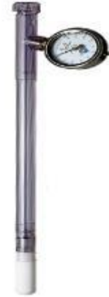
Tensiometers are useful for measuring soil moisture
